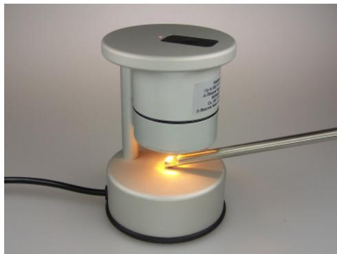
If the temperature of the instrument or of the endoscope is insufficient, the distance to the lamp can be varied. It's possible to run several switching cycles for example for larger instruments or other materials.
